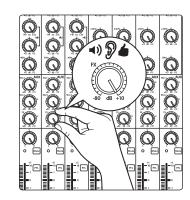
3. Use the FX send controls on each channel the same way that you use the faders to set the output level to your main mix. The higher a channel's level is in the effects mix, the more processed ("wetter") it will sound.
