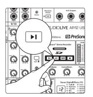
Press the Go to End button to advance playback to the end of the current 5. audio file. Press again to move to the end of the next file.
